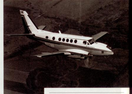
100 utilized the tail, landing gear, larger rudder, and shorter wings—with wing fences—of the Beech 99 airliner, as well as new fuel, pressurization, and heating systems.
